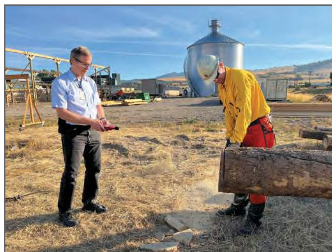
Figure 8—A team member capturing sound measurements while a sawyer makes a bucking cut.
