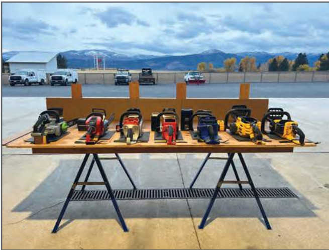
Figure 4—The seven test saws secured to a table in a covered outdoor setting.
